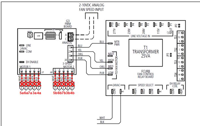
Figure 22 – Remove Motor Signal Wires
