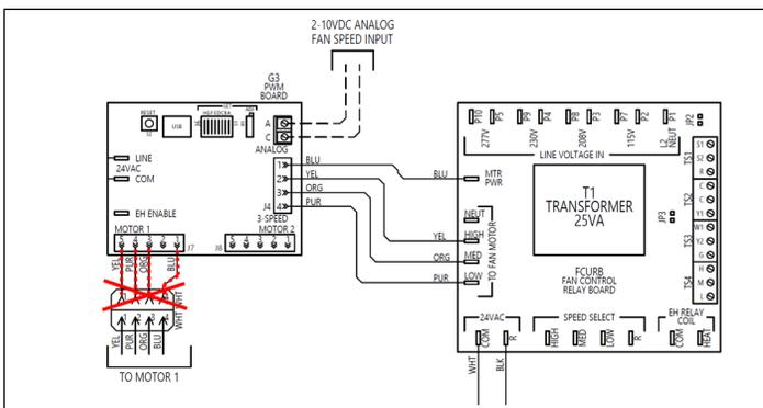
**Figure 50 – Remove Motor Signal Wires**
