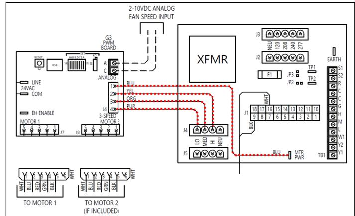
**Figure 30 – Remove low voltage signal wires to motor(s)**
