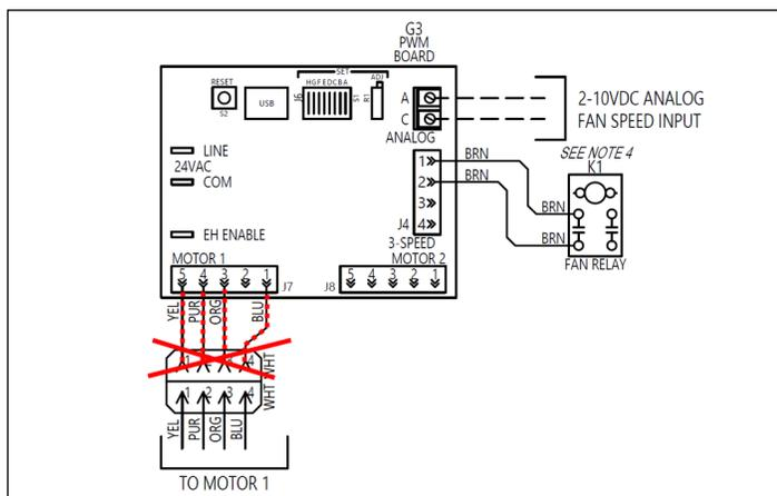
Figure 36 – Remove Motor Signal Wires
