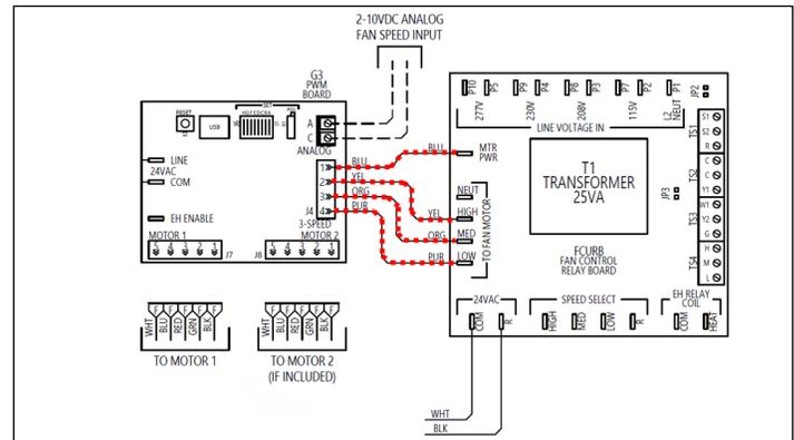
Figure 23 – Remove low voltage signal wires to motor(s)
