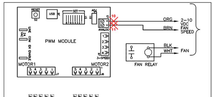
Figure 17 – Remove 2-10VDC motor control signal
