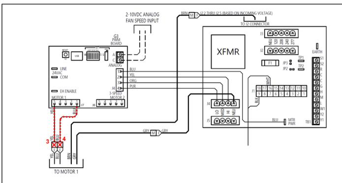
**Figure 64 – Remove Motor Signal Wires**
