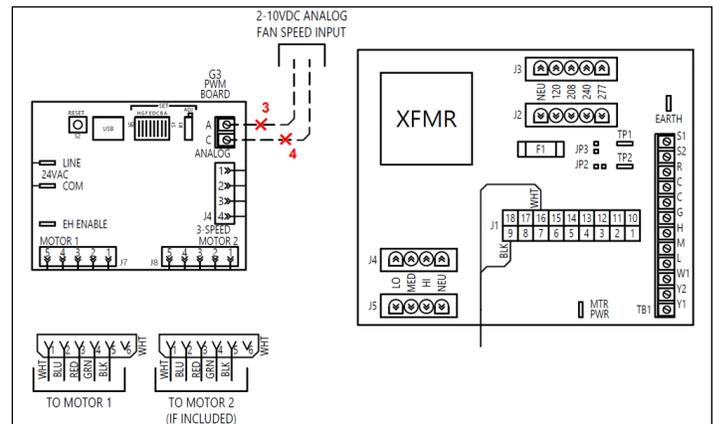
**Figure 31 – Remove 2-10VDC motor control signal**
