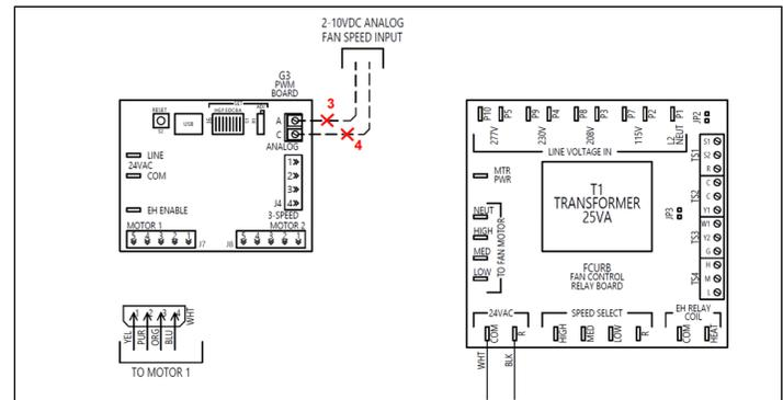
**Figure 52 – Remove 2-10VDC motor control signal**
