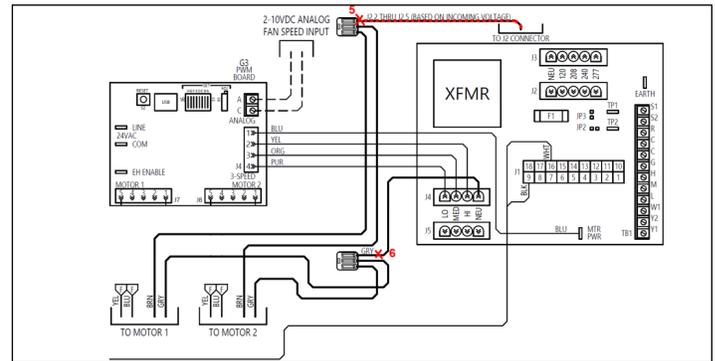
Figure 73 – Remove Motor Signal Wires
