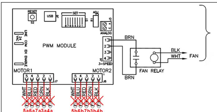
Figure 15 – Remove Motor Signal Wires
