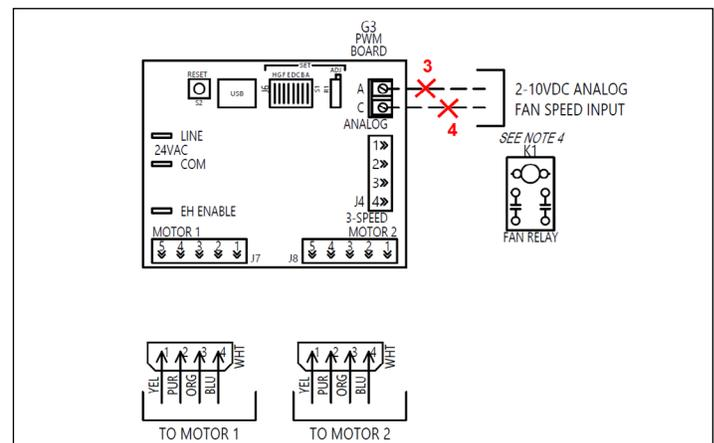
Figure 45 – Remove 2-10VDC motor control signal
