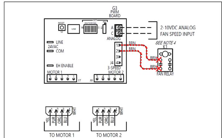
Figure 44 – Remove low voltage signal wires to motor(s)
