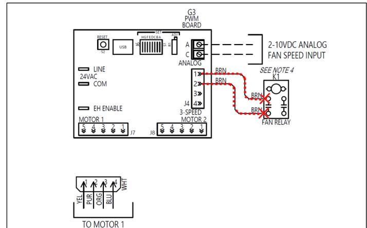
Figure 37 – Remove low voltage signal wires to motor(s)
