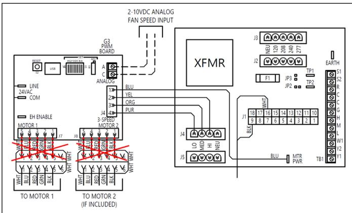
**Figure 29 – Remove Motor Signal Wires**
