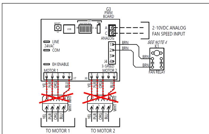
Figure 43 – Remove Motor Signal Wires
