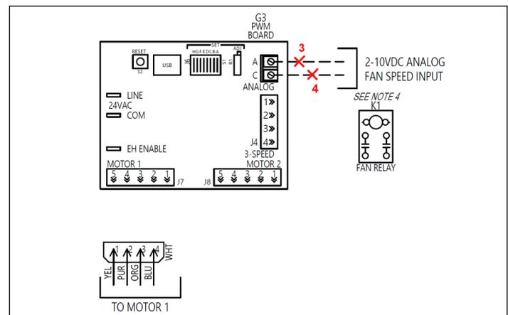
Figure 38 – Remove 2-10VDC motor control signal
