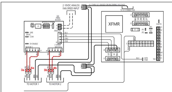
Figure 72 – Remove Motor Signal Wires
