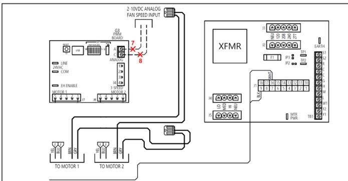
Figure 75 – Remove 2-10VDC motor control signal
