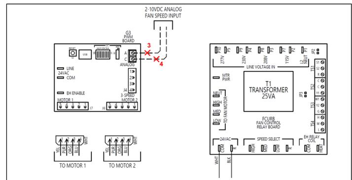
**Figure 59 – Remove 2-10VDC motor control signal**
