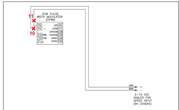
Figure 3 – Remove Motor Signal Wires
