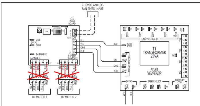
**Figure 57 – Remove Motor Signal Wires**
