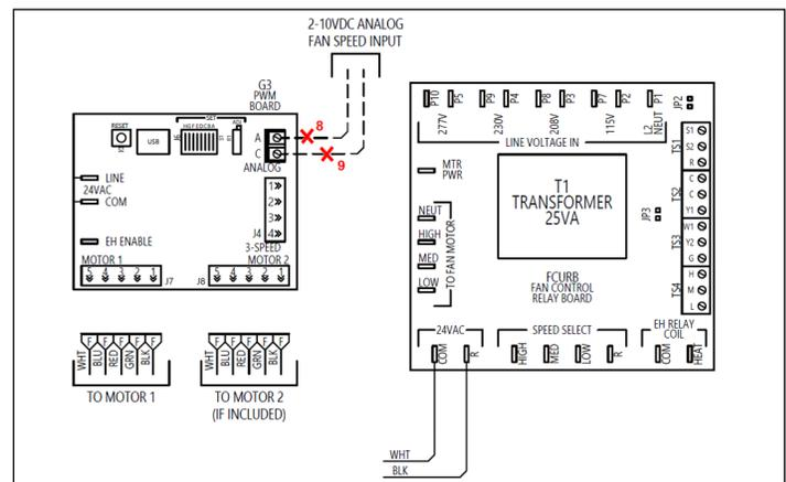
Figure 24 – Remove 2-10VDC motor control signal
