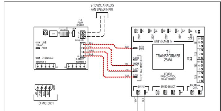
**Figure 51 – Remove low voltage signal wires to motor(s)**
