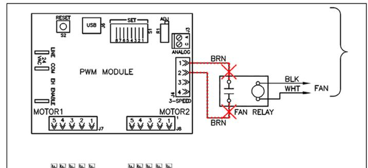
Figure 16 – Remove low voltage signal wires to motor(s)
