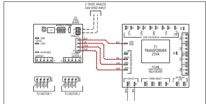
**Figure 58 – Remove low voltage signal wires to motor(s)**
